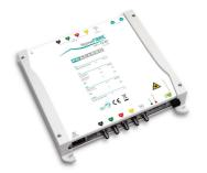
Optical transmitter for distribution of up to 4 satellites on a single fiber with CWDM (Coarse Wavelength Division Multiplexing) technology. **Innovative solution to transmit the entire TV band, including radio signals, and an entire orbital position** on a single fiber. **7dBm** with FP SAT+TV+FM laser, wavelength **1310nm**. (dimensions 230x230x50mm)
