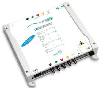
**Innovative solution that allows you to transmit the entire TV band, including radio signals, and an entire orbital position on a single fibre.** Optical transmitter suitable for CWDM (Coarse Wavelength Division Multiplexing) technology for the distribution of up to 4 orbital positions on a single fibre. Wavelength 1510nm, DFB at 7dBm (dimensions 230x230x50mm)
