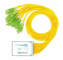
**32-way optical partition** suitable for building ROEs, with planar waveguide technology enabling **very low insertion losses**.
